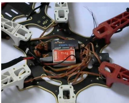
Figure 1 – Electrical part of the multicopter finished.
